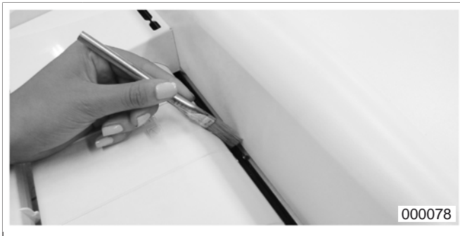
fig. 7 Cleaning the photocells
