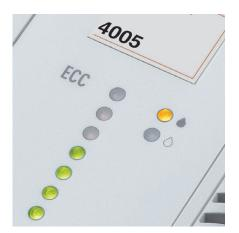
**ECC – ELECTRONIC CAPACITY CONTROL** This electronic feature indicates the used sheet capacity during shredding process to avoid paper jams.
